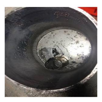
Figure 13: Liquid mercury found in equipment
